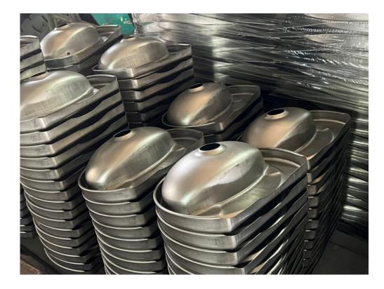
\*This image shows the working process of stainless steel wash basins. These wash basins are waiting to be lubricated and ground.
